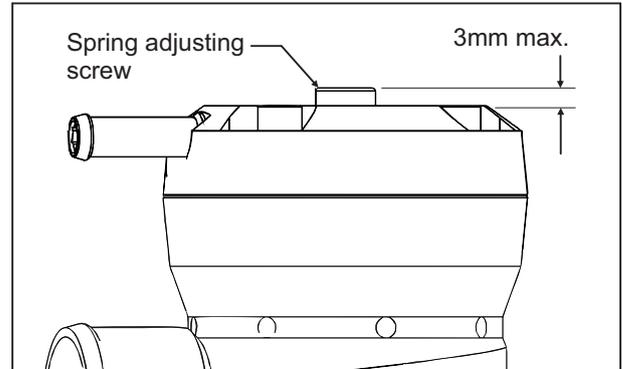
NOTE: On some cars, access to the adjustment screw is blocked by the ignition coil pack. In this case, it is easiest to loosen the valve mounting bolts 1 turn, then rotate the valve upwards just enough to make spring adjustments, then rotate the valve back down and re-tighten the mounting bolts.
